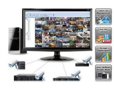
Intuitive liveview interface features user-defined display mode and advanced image rotation allowing users to design desired layout and freely rotate camera image to 90°, 180° or 270° degree. All the unique aspects of the site are able to plan on your liveview monitor design such as corridor, hall, etc.
